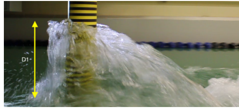
Figure 1: Measured maximum height of the bow wave ( D_1 ). Here the cylinder is towed from right to left.
