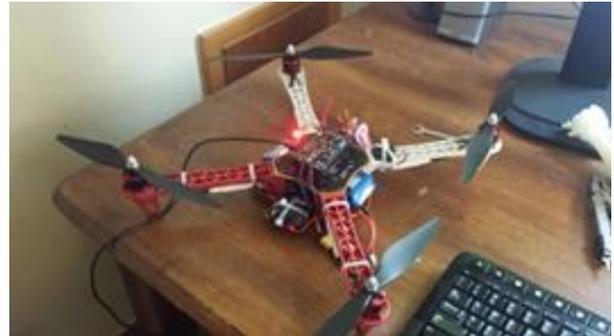
Figure 1: Quadrotor helicopter.
