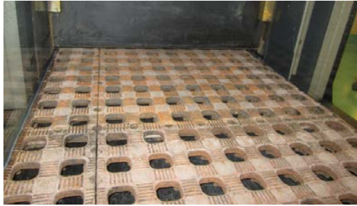
Figure 2. Bed roughness configuration; Note the sluice gate in the background
