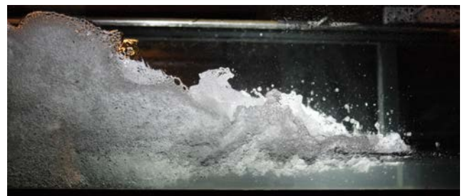
Figure 1. Laboratory hydraulic jump on smooth bed: Fr_1 = 4.5 ; Re = 1.8 \times 10^5 ; B = 0.5 m; d_1 = 0.055 m; x_1 = 1.25 m; flow from right to left
