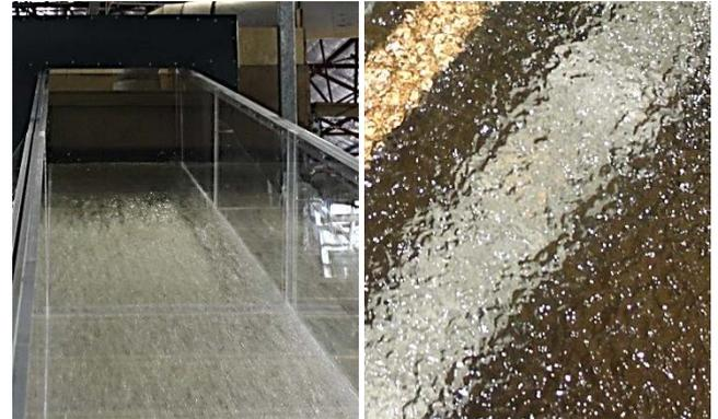
(A) Inception point of free-surface roughness (B) Top view of free-surface roughness
