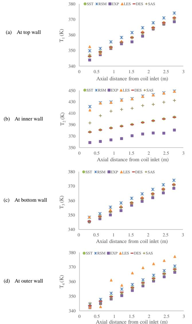
Figure 3. Wall temperature in the four circumferential locations.
