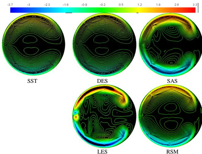
Figure 4. Helicity contours at pipe exit obtained from different models.
