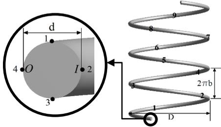
Figure 1. Schematic representation of the helical pipe indicating 4 circumferential thermocouples (left), 9 longitudinal locations (right).
