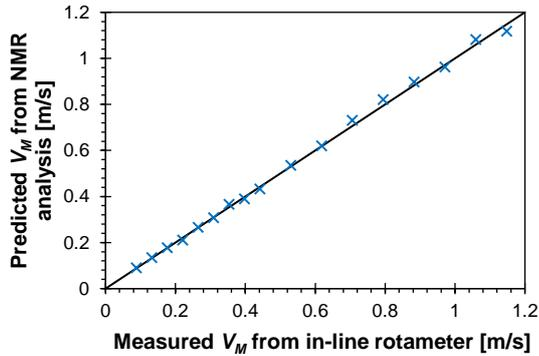
Figure 3. Comparison of the mean velocity ( $V_M$ ) predicted using regularisation of NMR data to the measured mean velocity from in-line rotameter data.
