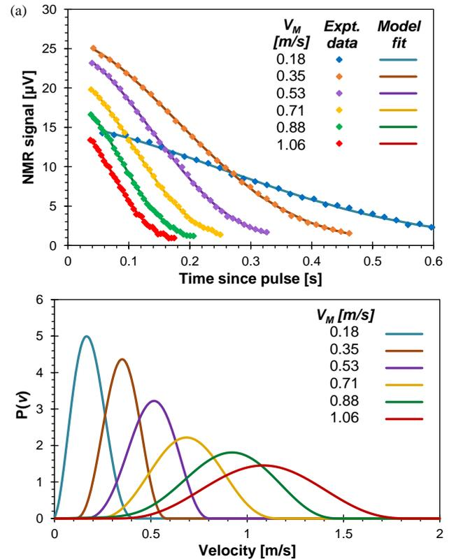
Figure 2. (a) Equation 1 fit to experimentally acquired FID data at mean velocities ranging from 0.18 to 1.06 m/s. (b) The corresponding velocity probability distributions returned by regularisation signal analysis.
