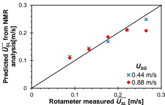
Figure 7. Comparison of NMR predicted mean superficial velocity to the measured mean superficial velocity from the in-line rotameter. Measurements were conducted at superficial liquid velocities of 0.09 – 0.26 m/s and superficial gas velocities of 0.44 and 0.88 m/s.
