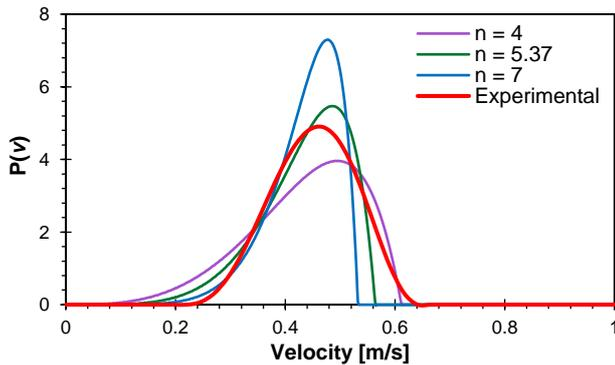
Figure 4. The experimentally obtained velocity distribution (at  $\bar{v} = 0.44$  m/s) compared to theoretical turbulent power law distributions. Power law exponents of  $n = 4$ , 5.37 and 7 are shown.
