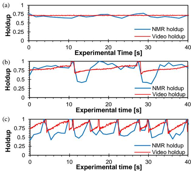
Figure 6. Tracking the instantaneous liquid holdup over time at superficial liquid velocities of; (a) 0.09 m/s (stratified flow), (b) 0.18 m/s (slug flow) and (c) 0.26 m/s (slug flow). The liquid holdup as determined by NMR signal analysis is compared to the holdup estimated from video analysis.
