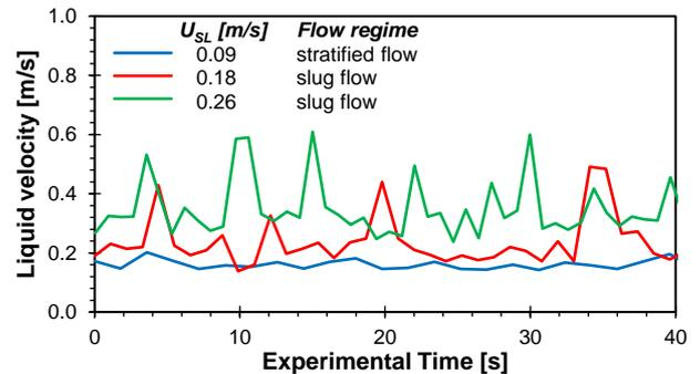
Figure 5. Tracking the instantaneous liquid velocity over time at superficial liquid velocities of 0.09, 0.18 and 0.26 m/s respectively and at a gas superficial velocity of 0.44 m/s. The visually observed flow regime is indicated for each superficial liquid velocity.
