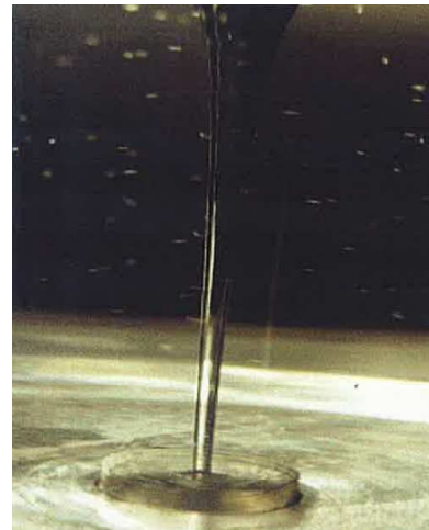
Figure 1: Photo taken in experiments with bathtub vortex on a rotating table [2].
