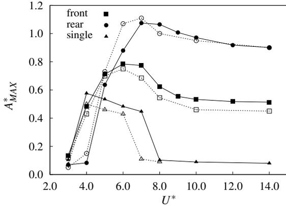
Figure 3: For  $T = 0.0$  and  $L = 1.5$ , the variation with  $U^*$  of the maximum displacement of the each cylinder. Solid symbols represent results from the current study, while hollow ones are from Borazjani and Sotiropoulos [2].
