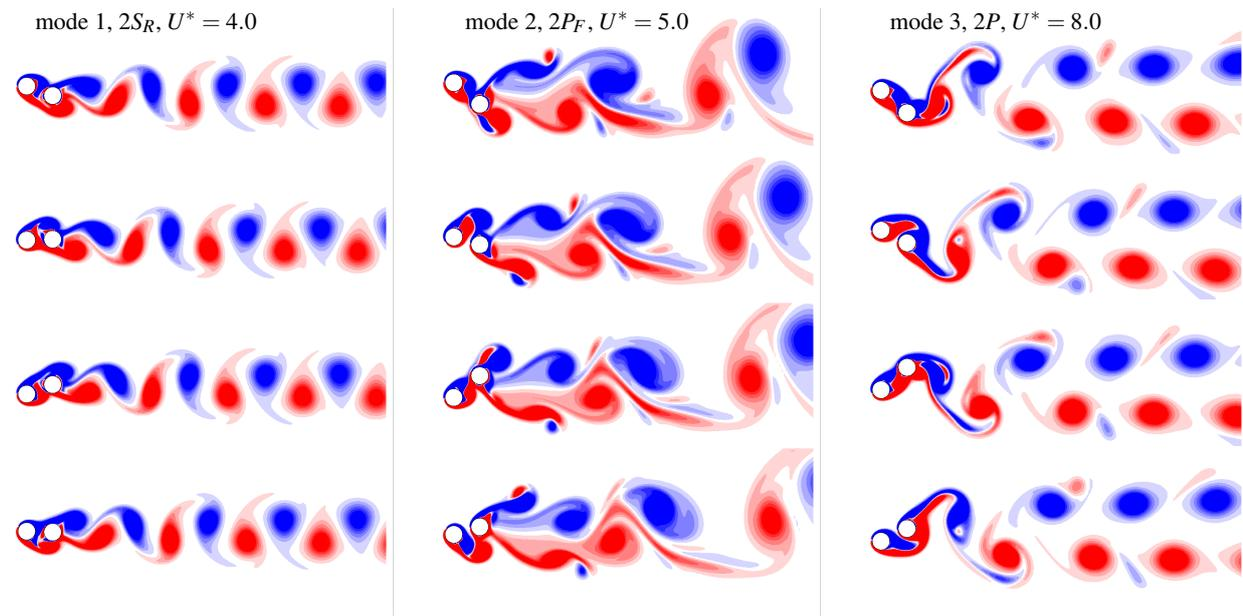
Figure 4: For the tandem cylinder arrangement ( $T = 0$ ), vorticity contours for three cases,  $U^* = 4.0, 5.0$  and  $8.0$ , describing the three vortex-shedding modes,  $2S_R$ ,  $2P_F$  and  $2P$ . Each series of images depicts an entire oscillation cycle, beginning with the front cylinder at its maximum displacement. Contours vary in the range  $-1 \leq \omega_z \leq 1$ .
