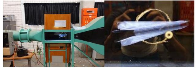
Figure 4. Experimental setup of Hexafly smoke tunnel model.
