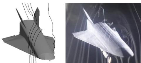
Figure 9. Asymmetric vortex in CFD (left) and smoke tunnel (right).
