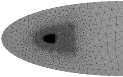
Figure 1. Half body mesh typical of the Michigan AFRL cruiser and Hexafly-Int vehicles containing approximately  $15 \times 10^6$  elements.
