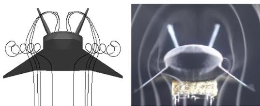
Figure 8. Comparison of vortex behaviour for Hexafly-Int Vehicle seen in CFD (left) and smoke tunnel (right) at 15 degrees  $AoA$ .
