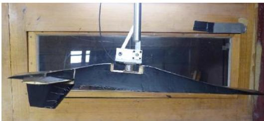
Figure 3. Experimental setup of 3x4 ft Michigan AFRL cruiser wind tunnel model.
