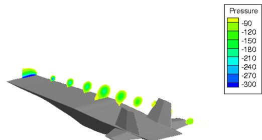
Figure 11. Vortex formation and fin interaction of Michigan AFRL cruiser (right) at 10 degrees  $AoA$ .
