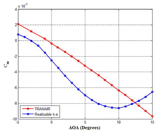
Figure 6. CFD and TRANAIR results of Hexafly  $C_m$  vs  $AoA$ .
