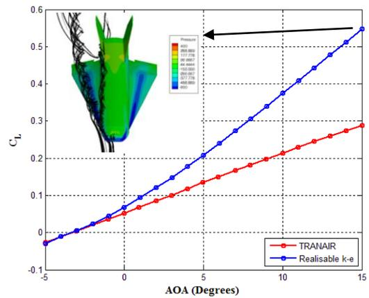
Figure 5. CFD and TRANAIR results of Hexafly  $C_L$  vs  $AoA$  showing strong leading edge vortices for the 15 degree  $AoA$  case.
