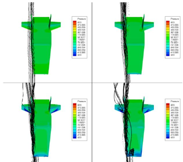
Figure 10. Michigan AFRL Cruiser vortex formation at (a) 0 degrees  $AoA$  (top left), (b) 5 degrees  $AoA$  (top right), (c) 10 degrees  $AoA$  (bottom left) and (d) 15 degrees  $AoA$  (bottom right).
