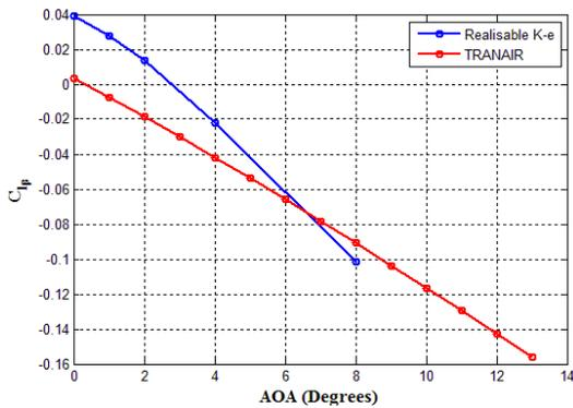
Figure 7. CFD and TRANAIR results of Hexafly roll moment coefficient gradient for increasing  $AoA$ .
