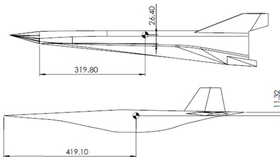
Figure 2.  $CoG$  location for Hexafly-Int (top) and AFRL Cruiser (bottom)
