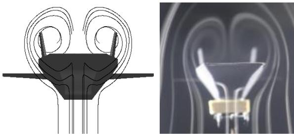
Figure 13. Comparison of vortex behaviour for Michigan AFRL cruiser seen in CFD (left) and smoke tunnel (right) at 15 degrees  $AoA$ .
