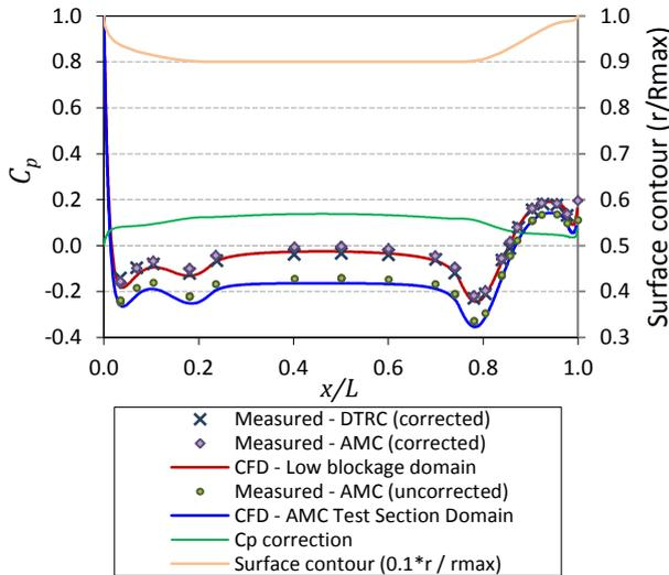
Figure 5. Surface pressure coefficient ( $C_p$ ) distribution for the SUBOFF hullform: AMC test section domain (CFD), low blockage domain (CFD), DTRC [3] (measured, uncertainty = 0.015) and AMC [1] (measured, uncertainty 0.007) at  $Re = 12 \times 10^6$ .
