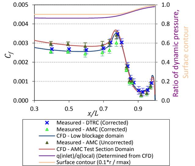
Figure 6. Skin friction results contrasting the CFD calculations to the original DTRC SUBOFF measurements [3] and the AMC experimental data [1] at  $Re=12 \times 10^6$ . The surface contour of the SUBOFF hullform and the ratio of dynamic pressure,  $q(inlet)/q(local)$ , is also included for reference.
