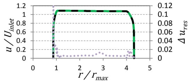
Figure 3. Normalised mean velocity as a function of normalised radius for the two finest meshes, along a line  $135^\circ$  from the spanwise direction of the support foils for the SUBOFF hullform at a longitudinal position of  $x = 0.7 L$  along the model. Results from the high resolution mesh,  $u_{hi}$ , are shown by the green line and results from the second finest resolution mesh,  $u_{mh}$ , by the black dashed line. The purple dots represent  $\Delta u_{res}$  for the second finest mesh.
