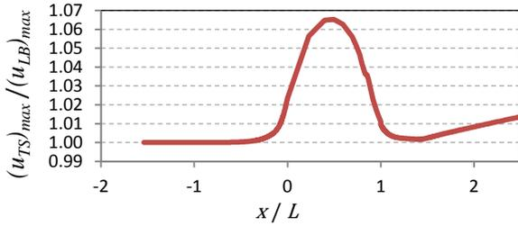
Figure 4. The maximum velocity ratio of the AMC test section domain,  $u_{TS}$ , to the low blockage domain,  $u_{LB}$ , for the SUBOFF hullform. The horizontal axis is normalised by the length of the SUBOFF model, where  $x = 0$  is at the tip of the model nose.
