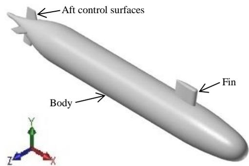
Figure 1. Fully appended SUBOFF generic nuclear submarine hullform.
