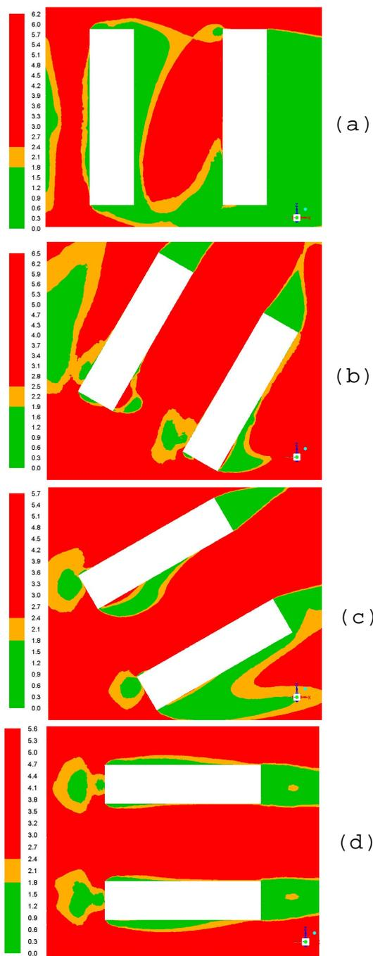
Figure 3: Velocity magnitude (m/s) contours in XZ- plane at pedestrian level height (1.75m) for angle of attack (a)  $0^\circ$  (b)  $30^\circ$  (c)  $60^\circ$  (d)  $90^\circ$ , green represents 0 to 1.8 m/s (which can be considered a comfort zone for pedestrians), orange represents 1.81 to 2.4 m/s (zone in which the wind starts causing impact on people). Red represents wind speeds above 2.4 m/s.
