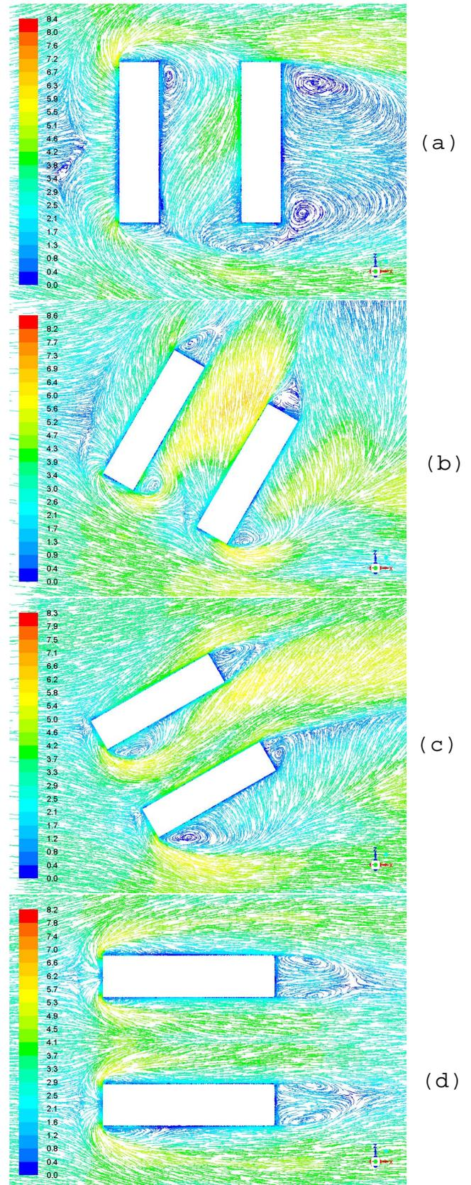
Figure 2: Velocity magnitude (m/s) pathlines in XZ- plane at pedestrian level height (1.75m) for angle of attack (a)  $0^\circ$  (b)  $30^\circ$  (c)  $60^\circ$  (d)  $90^\circ$ .
