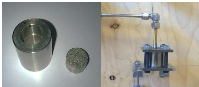
Figure 2. Combustion chamber with sintered steel porous insert (left) and rig setup (right)
