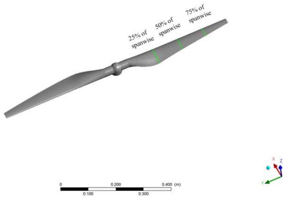
Figure 2: solid 3D model of tidal turbine blades
