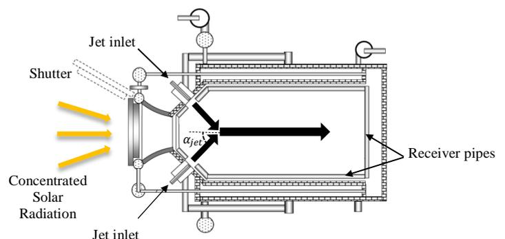
Figure 1. Hybrid Solar Receiver Combustor [11].
