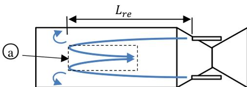
Figure 5. Flow regime 1 (a = annular inward recirculation,  $L_{re}$  = recirculation length).
