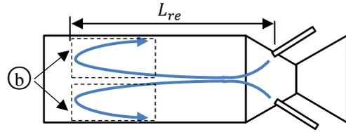
Figure 6. Flow regime 2 (b = annular outward recirculation).
