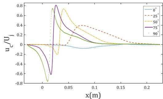
Figure 9. Calculated evolution of the axial velocity  $u_c$  along the HSRC centreline normalised by injection velocity  $U_j$  as a function of the HSRC length for five inclination angles,  $x = 0$  m refers to the location of the aperture plane. The range of  $x < 0$  m refers to the secondary concentrator.
