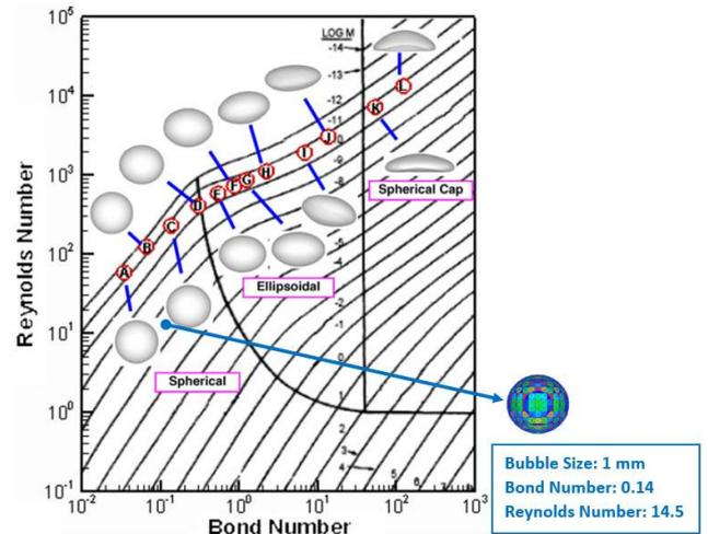
Figure 8. Comparison of 1 mm bubble shape using the ISM method with Hua et al.'s numerically predicted terminal bubble shapes [9].
