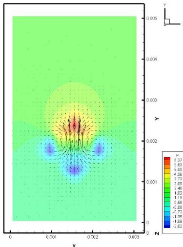
Figure 6. Pressure field plot with velocity vectors (Axes denote physical geometries [m], Pressures are in Pascals).
