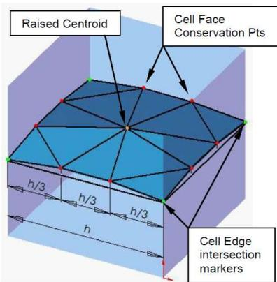
Figure 1. InterSection Marker (ISM) representation of a 2D interface in a rectangular hexahedral control volume.
