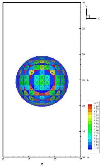
Figure 4. Surface Plot, control volume width = 0.1 mm (Axes denote control volumes [-]). Simulation time = 0.00975 sec.
