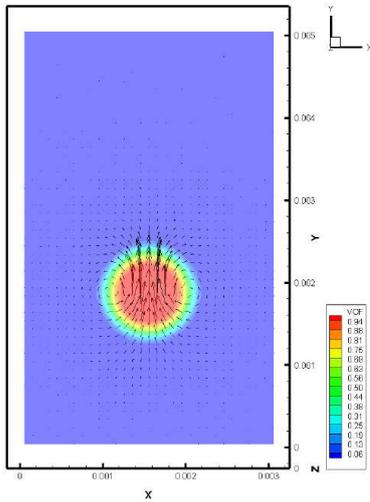
Figure 5. Distributed VOF plot with velocity vectors. (Axes denote physical geometries [m]).
