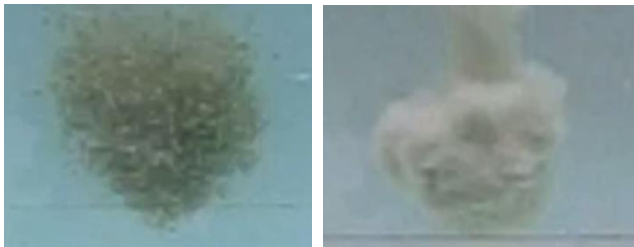
Figure 3: Spherical 'blob' observed during underwater dispersion for W6 sand (left) and W9 sand (right).
