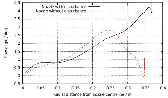
Figure 4. Comparison of exit flow angle distributions for Mach 12 nozzles with and without centreline disturbances
