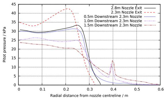
Figure 6. Pitot pressure distributions at different nozzle exit stations and downstream locations in the dump-tank
