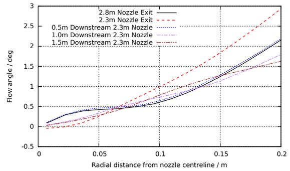
Figure 7. Flow angle distributions at different nozzle exit stations and downstream locations in the dump-tank
