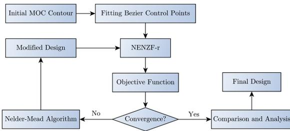
Figure 1. Work flow for the CFD-based computational optimisation design
