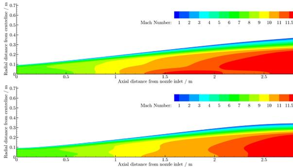
Figure 2. Mach number contours of Mach 12 nozzles with (top) and without (bottom) centreline disturbances
