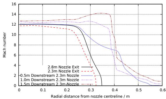
Figure 5. Mach number distributions at different nozzle exit stations and downstream locations in the dump-tank
