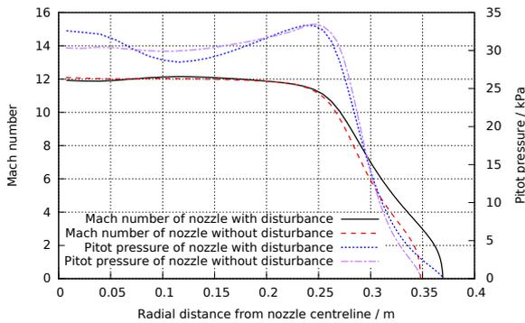
Figure 3. Exit Mach number and Pitot pressure distributions for Mach 12 nozzles with and without centreline disturbances
