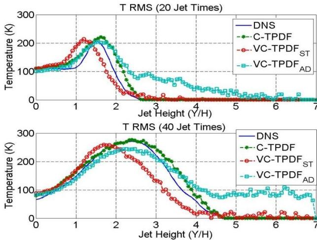
Figure 8. RMS temperature profile at 20 and 40 jet times for DNS, C-TPDF and VC-TPDF models.
