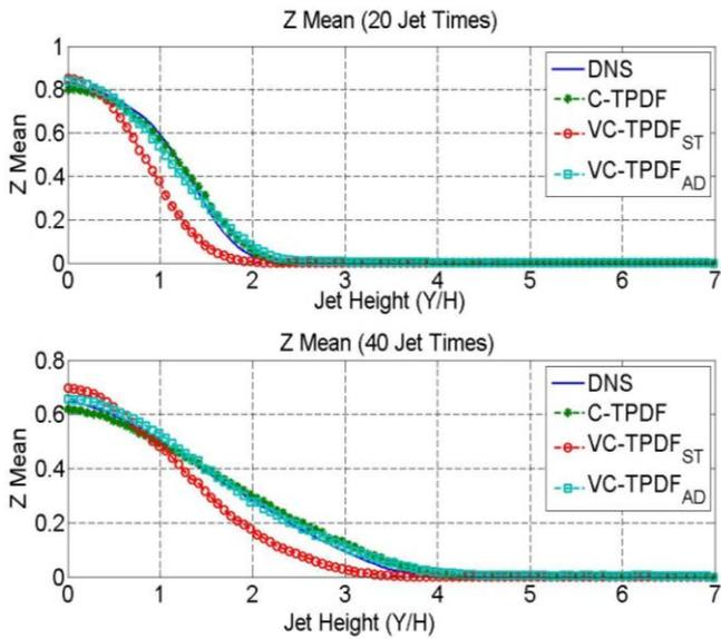
Figure 3. Mean mixture fraction profile at 20 and 40 jet times for DNS, C-TPDF and VC-TPDF models.
