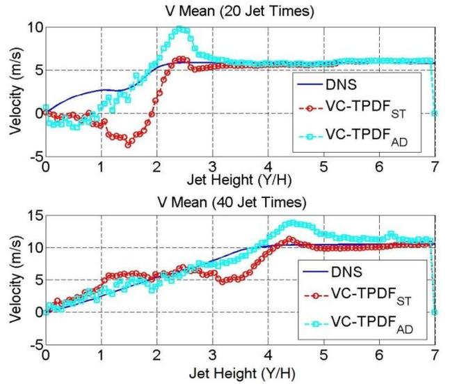
Figure 5. Mean velocity profile at 20 and 40 jet times for DNS, C-TPDF and VC-TPDF models.
