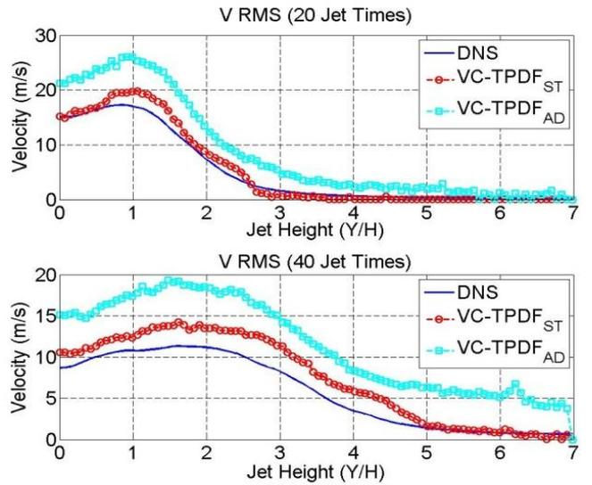
Figure 6. RMS velocity profile at 20 and 40 jet times for DNS, C-TPDF and VC-TPDF models.
