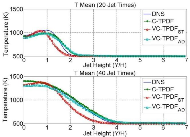
Figure 7. Mean Temperature statistics at 20 and 40 jet times for DNS, C-TPDF and VC-TPDF models.
