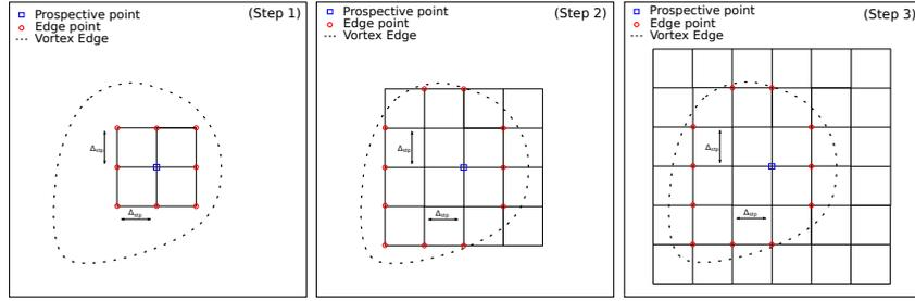
Figure 3: Vortex edge and center detection example.
