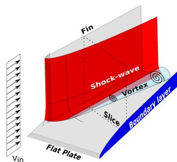
Figure 1: Flat plate and fin vortex generation.
