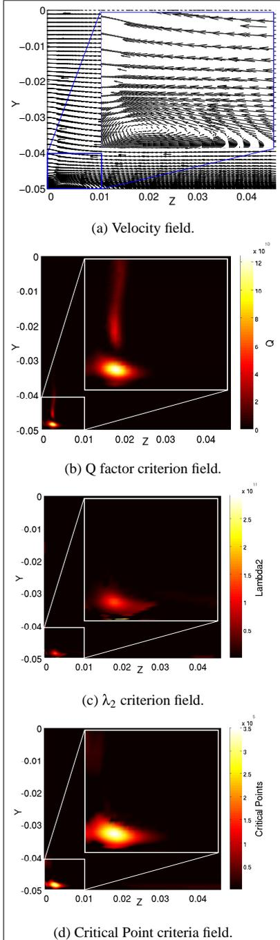
Figure 4: Velocity and criteria fields on a single slice from the simple geometry 45.0mm downstream of the fin leading edge and with its normal forming a  $20^\circ$  angle with the axial direction.
