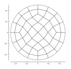
Figure 1: Distribution of spectral elements within the pipe cross section
