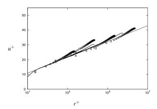
Figure 3: Pipe flow mean streamwise velocity profiles. Squares: LES; solid line: experiment McKeon *et al.* [10] at  $Re_{\tau} = 1.8 \times 10^3, 2.0 \times 10^4, 2.2 \times 10^5, 5.3 \times 10^5$ ; dashed line: log-law with  $\kappa = 0.43$  and B = 5.5, obtained from LES.
