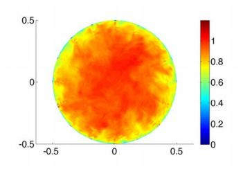
Figure 4: Instantaneous color-coded image of the instantaneous stream-wise velocity component.  $Re_{\tau} = 2 \times 10^5$ .
