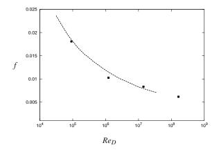
Figure 2: Friction factor f versus  $Re_b$ . Squares: LES; dashed line: experimental result of McKeon *et al.* [9].
