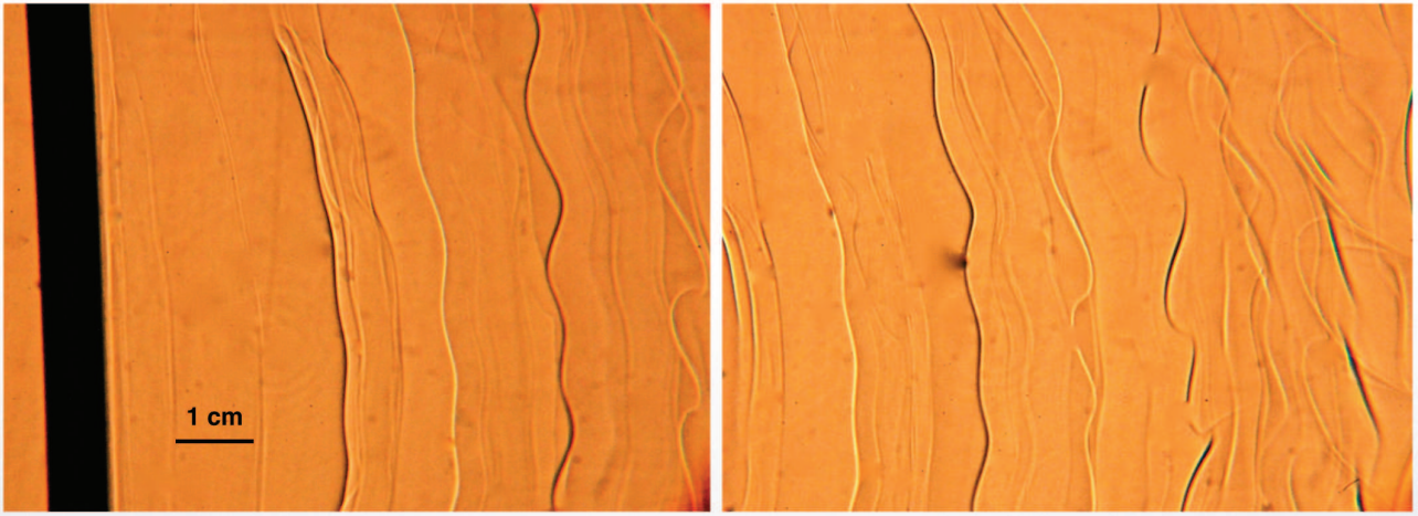
Figure 3: Shadowgraph sideview visualizations of the mode S: the wake behind a cylinder is tilted at \alpha = 45^\circ for Re = 170 and F = 2.5 . The cylinder is going to the left of the picture and there is a time delay of approximately 7 D/U between both pictures to reveal the temporal evolution of the instability. The field of view is approximately 8 by 15 diameters.
