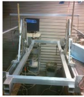
Figure 3. David Cox’s hot wire cutting machine.
