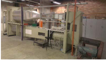
Figure 2. Closed loop wind tunnel located at the University of Technology, Sydney (UTS).
