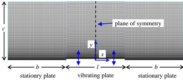
Figure 1. Physical geometry and computational domain.
