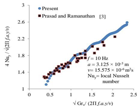
Figure 2. Comparison of computational results with the experimental results of Prasad and Ramanathan [3].
