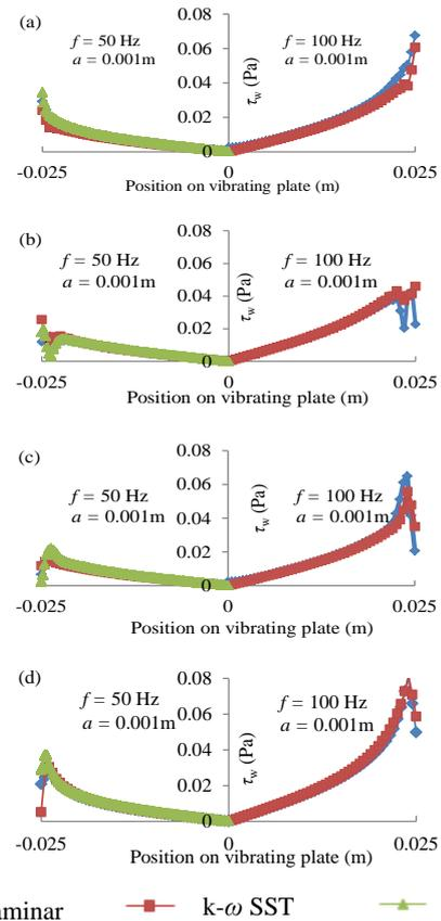
Figure 4. Local wall shear stress (instantaneous) illustrated at various phases of the cycle of vibration (a) 25 %; (b) 50 %; (c) 75 %; (d) 100 %.
