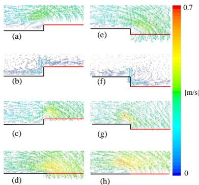
Figure 3. Velocity vectors (coloured by velocity magnitude) in the vicinity of the vibrating plate at different phases of a cycle of vibration. (a) 12.5 % (b) 25 %; (c) 37.5 %; (d) 50 %; (e) 62.5 %; (f) 75 %; (g) 87.5 %; (h) 100%.
