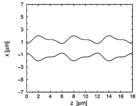
Figure 2. Schematic of the profile (along the pore axis – z-axis) of a drift ratchet studied by Kettner et al. [7].
