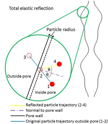
Figure 4. Schematic of how the particle-wall interactions are represented in the model currently being developed. The length of points 2-3 and 2-4 are equal.
