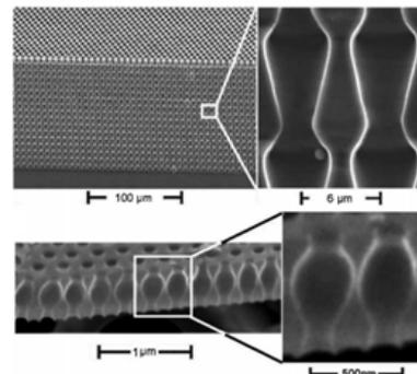
Figure 3. (Top) SEM of a massively parallel silica membrane with asymmetric pores [11]. (Bottom) SEM of girdle band pores of diatom *Coscinodiscus sp.* [9].
