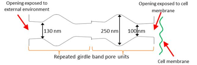
Figure 6. Schematic of the profile (along the pore axis) of the girdle band pores of the diatom *Coscinodiscus sp.*
