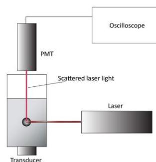
Figure 1. Set-up for measuring the SBSL intensity and radial dynamics from Leong et al. [10] Copyright (2014) by the American Physical Society.
