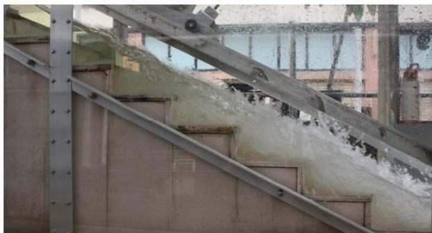
Figure 1. Air-water flows downstream of the inception point of free-surface aeration on a stepped spillway ( $\theta = 26.6^\circ$ ); skimming flow regime;  $d_c/h = 1.25$ ,  $q_w = 0.137 \text{ m}^3/\text{s}$ ,  $Re = 5.5 \times 10^5$
