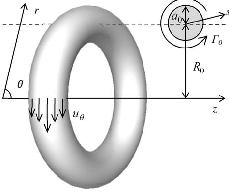
Figure 1. Schematic of the axisymmetric coordinate system for a swirling ring.  $R_0$ ,  $a_0$ ,  $\Gamma_0$  and  $v_\theta$  are flow parameters, while  $z$ ,  $r$ ,  $\theta$ , and  $s$  are coordinate descriptors. The vorticity and swirl profiles of the vortex core are both initially Gaussian.
