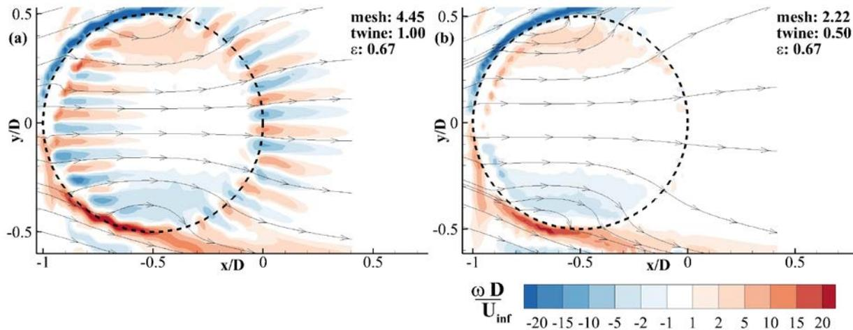
Figure 1: Time averaged vorticity distribution and stream lines around two models of same porosity ( $\epsilon = 0.67$ ) but varying mesh and twine size (a) mesh = 4.45 mm and twine = 1.00 mm (b) mesh = 2.22 mm and twine = 0.50;  $Re = 900$ .
