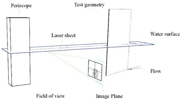
Figure 2. Experimental setup schematic for towing tank carriage mounted PIV
