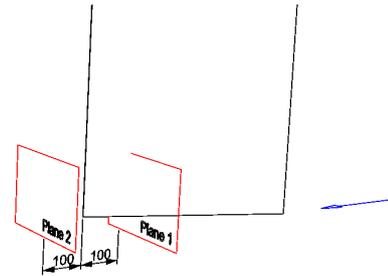
Figure 3. Position of planes captured in relation the trailing edge datum using 2D PIV.
