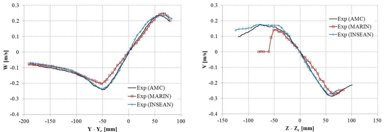
Figure 7. Experimental results from the HTA and AMC showing the magnitude of the W and V vectors with reference to the vortex centre.
