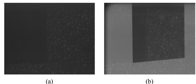
Figure 4. Double frame raw images from measurement plane 1 showing the absence of reflection from the test geometry and dense high contrast seeding (a) First pulse and (b) Second pulse
