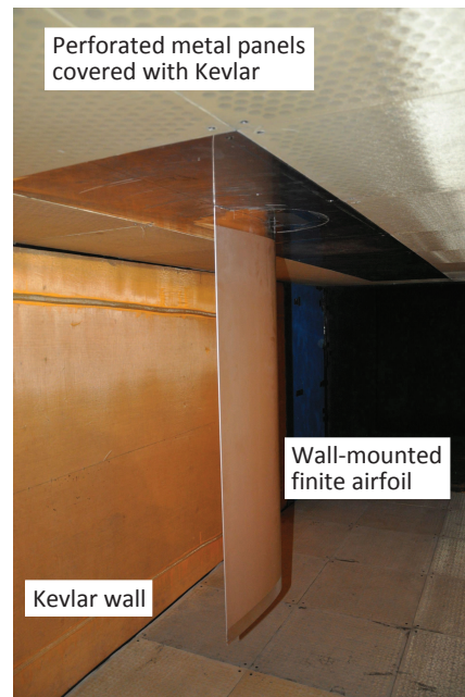
Figure 3. The wall-mounted finite airfoil model in the Stability Wind Tunnel anechoic test section.
