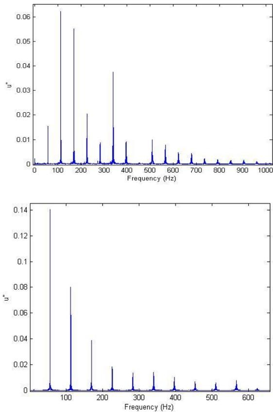
Figure 4. Frequency spectrum of the streamwise fluctuation ( $u''$ ) at the upwash region; from top to bottom: At  $y/\delta_L=0.25$ ; At  $y/\delta_L=0.5$ ; At  $y/\delta_L=0.75$ ; d. at  $y/\delta_L=1$ ; where  $\delta_L$  is the local Blasius Boundary layer thickness.
