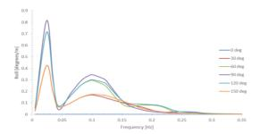
Figure 9. Roll RAO curves for various wave headings
