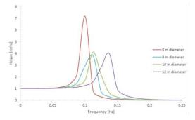
Figure 4. Heave RAO curves for various diameter columns
