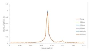
Figure 11. Heave amplitudes in frequency domain for various wave directions
