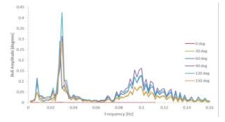
Figure 13. Roll amplitude s in frequency domain for various wave headings
