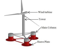
Figure 1. Geometry of the FOWT design
