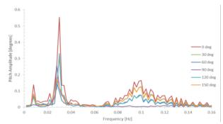
Figure 12. Pitch amplitude s in frequency domain for various wave headings
