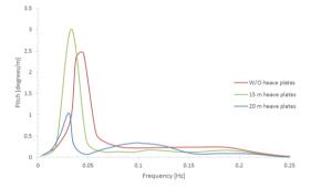
Figure 6. Pitch RAO curves for various heave plate sizes
