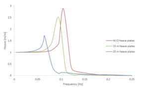
Figure 5. Heave RAO curves for various heave plate sizes
