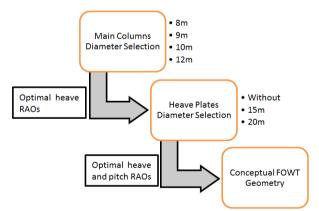
Figure 2. Geometry selection procedures
