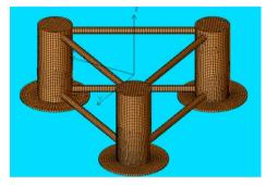
Figure 3. Meshed FOWT foundation structure
