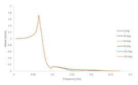
Figure 7. Heave RAO curves for various wave headings
