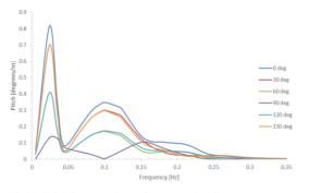
Figure 8. Pitch RAO curves for various wave headings
