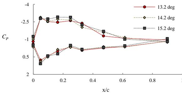
Figure 5. Pressure distribution for the NACA 0021 airfoil at angles when the lift curve has levelled off. The airfoil is pitching at  $\kappa = 0.024$ .
