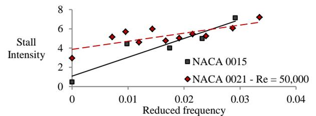
Figure 7. Effects of increasing reduced frequency on the stall intensity factor of two different airfoils (NACA 0015 from Jumper et al. (1987b) and the NACA 0021 from current experiments).
