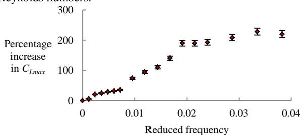
Figure 6. Percentage increase in the maximum lift as a function of reduced frequency at a Reynolds number of 50,000.
