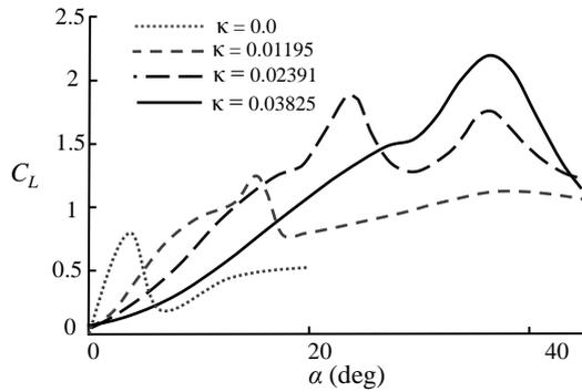
Figure 2. Dynamic stall lift characteristics as a function of reduced frequency ( $Re = 50,000$ ) for the NACA 0021 airfoil.
