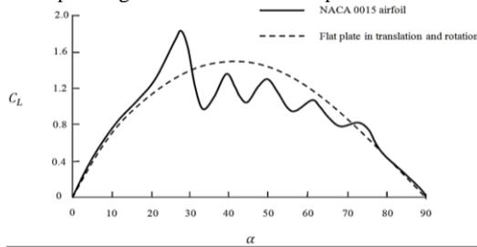
Figure 8 - Lift coefficient for a pitching 0015 airfoil [24] and a flat plate undergoing both rotation and translation [25], showing similar parabolic trend.
