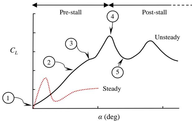
Figure 3. Schematic illustration and the stages of the lift-curve for an airfoil undergoing dynamic stall.
