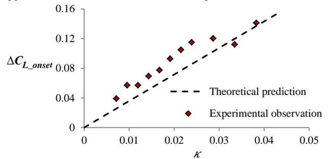
Figure 4. Comparison of theoretical lift prediction at the onset and the experimental observation for the 0021 airfoil.
