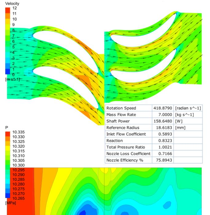
Figure 4. Water flow simulation through small turbodrill model with mass flow rate of 7 Kg/s and rotation speed of 4,000 rpm.
