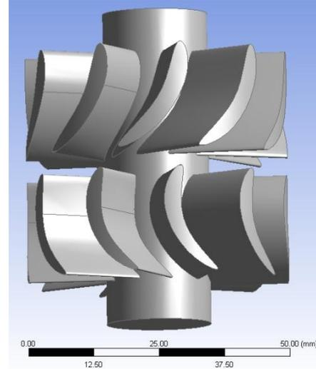
Figure 2. Geometry model of the one stage turbodrill with 10 blades on each row.
