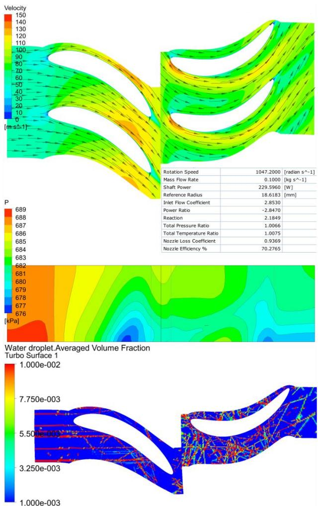
Figure 6. Two phase flow (mist) simulation of air (0.1 Kg/s) as continuous phase and water droplets (0.1 Kg/s) as dispersed fluid particle.
