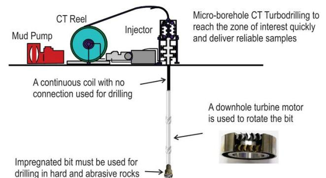
Figure 1. Schematic of a coiled tubing unit with main assembly proposed for hard rocks mineral exploration drilling.
