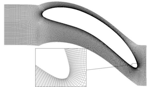
Figure 3. Blade to blade view of the high quality hexahedral mesh for the stator at mid-span.
