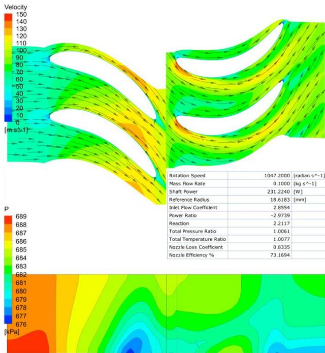
Figure 5. Air flow simulation through small turbodrill model with mass flow rate of 0.1 Kg/s, and rotation speed of 10,000 rpm.
