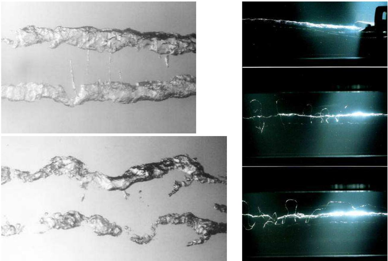
Figure 1: Images of cavitation in vortical flows.
