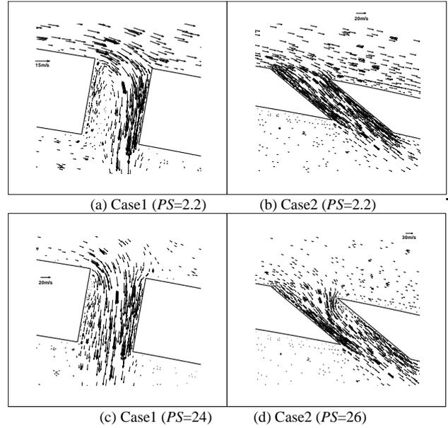
Fig.5 Velocity vector field of injection holes
