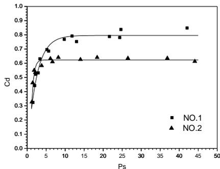
Fig.4 Curves of discharge coefficient with  $PS$
