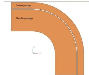
Fig. 3 Model of computation domain
