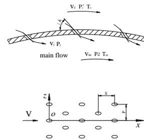
Fig.1 Discrete-hole curved wall scheme
