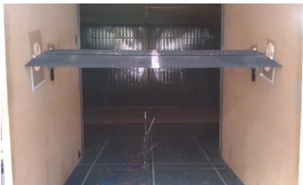
Figure 2. This figure shows the test model mounted horizontally in the TFWT with contraction in place. The Pitot - static tube in front of the wings measures the reference static and dynamic pressure to convert values to coefficients
