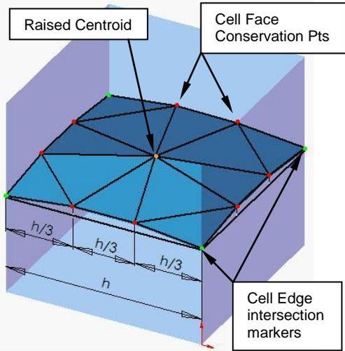
Figure 1. Intersection-marker (ISM) representation of a 2D interface in a regular hexahedral control volume.
