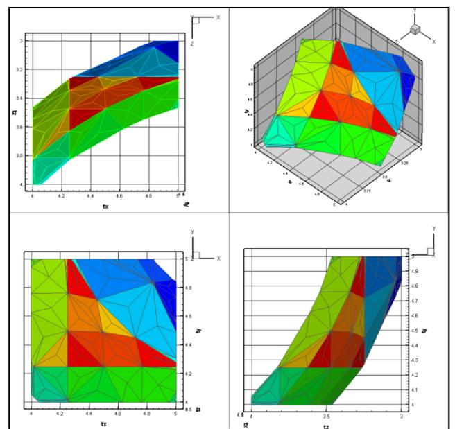
Figure 5: Typical composite interface within a control volume before remeshing
