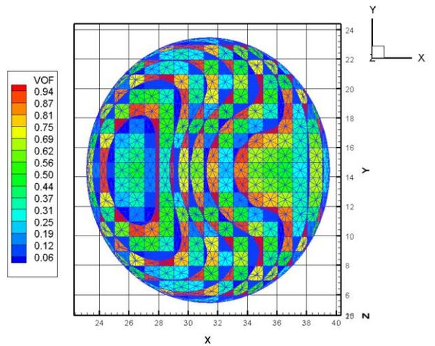
Figure 8. Top view of RBC mapped to CFD mesh showing each interface clearly within the bounds of its own control volume.
