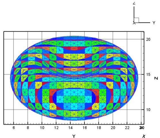
Figure 9. Front view of RBC interface model in finite volume mesh.
