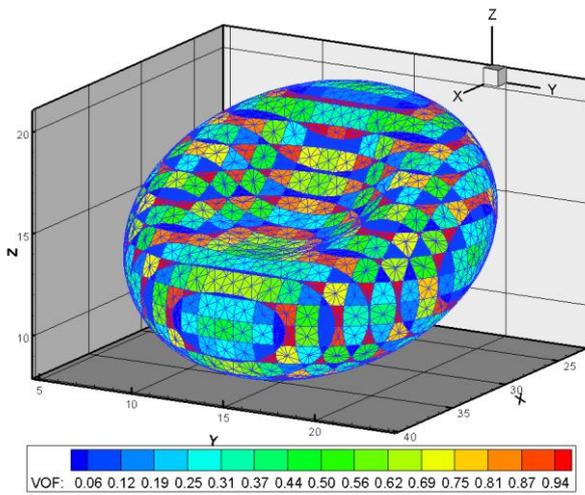
Figure 6. 2D Interface tracking of a disc-shaped RBC inside regular cube mesh. Compound curvatures inside unit-volume mesh are displayed in Volume of Fraction (VOF) contours.
