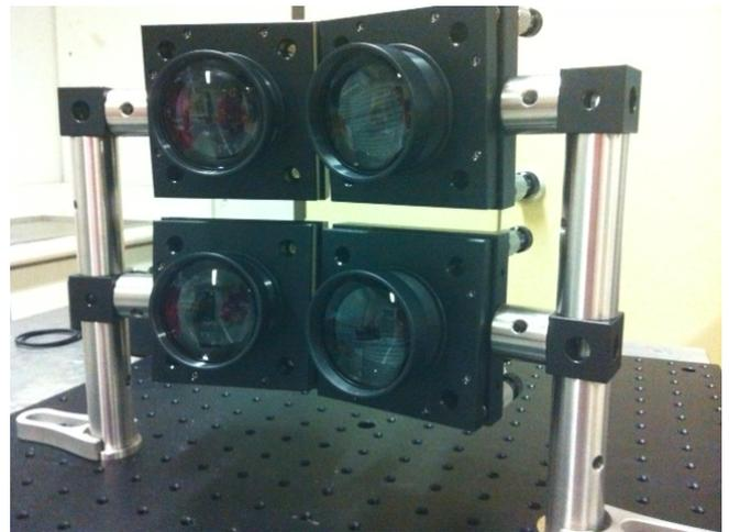
Figure 1: Pyrometer front, showing 2  $\times$  2 arrangement of lenses. Filters and detectors are connected behind lenses.
