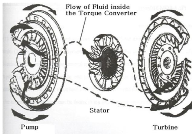
Figure 1. Torque converter fluid flow path [9].
