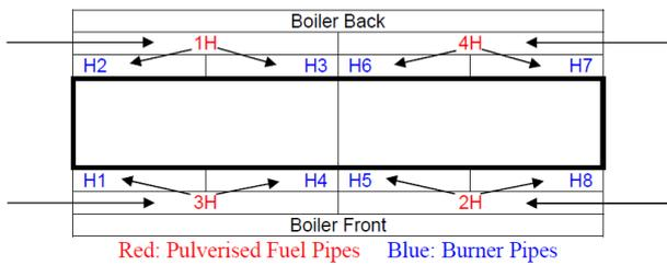
Figure 3. Layout and labelling of pipes from the 1H-pulveriser mill [1].
