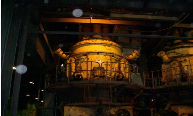
Figure 2. Photo of a coal pulveriser mill.
