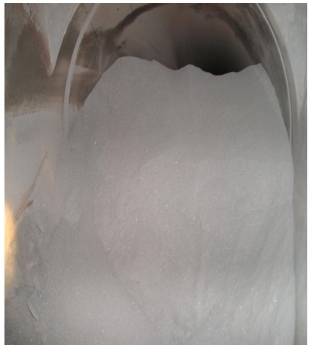
Figure 1. Deposits in a coal-fuel pipe.
