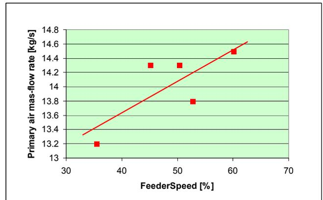
Figure 10. Primary air mass-flow rate versus feeder speed (fraction of coal-feed speed corresponding to operating capacity). Raw data from [1].
