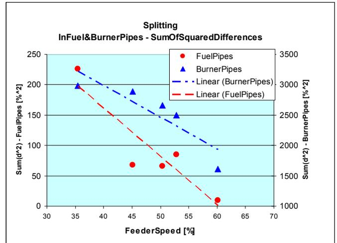
Figure 9. Reduction in the fuel flow distributions in the pipes; sum of squared deviations from desired distributions (25% in pulverised-fuel pipes, 50% in burner pipes); feeder speed is in % of full-capacity speed which corresponds to 45 tonnes/hr of coal. Raw data from [1].
