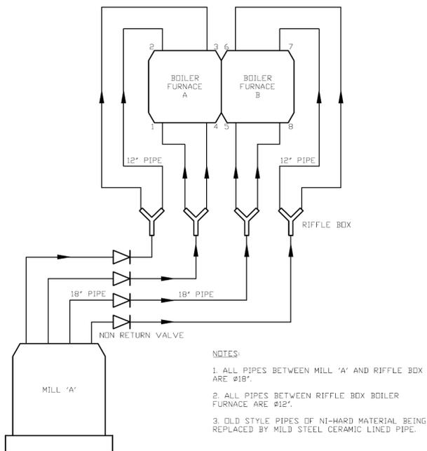
Figure 4. Schematic of a pipe-network from a pulveriser mill to a boiler; pulverised-fuel or mill pipes are before the rifle box, burner pipes after; all 8 burner pipes connect to the boiler at a same elevation.
