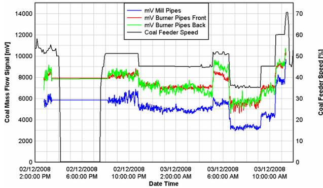
Figure 7. Measured total coal flow signals and DCS (distributed control system) coal feeder speed (as percent of mill operational speed) [1].
