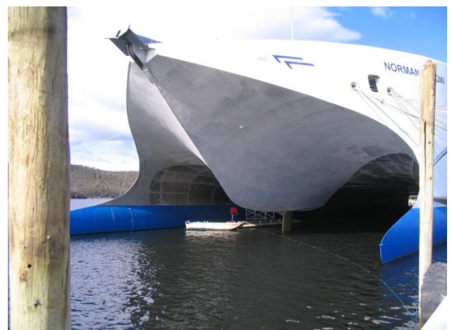
Figure 1. INCAT Tasmania 112m Wave Piercing Catamaran, showing centre bow keel and demi-hull bows (both will be on the water line when loaded).
