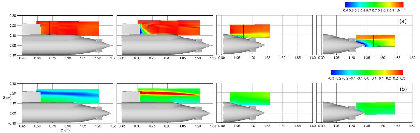
Figure 7. Ensemble-averaged non dimensional (a) stream-wise velocity, and (b) transverse velocity. Measurement planes MP1 to MP4 are shown from left to right
