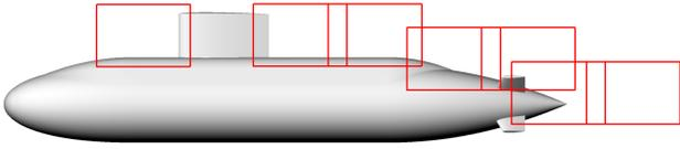
Figure 2. Locations of PIV measurement field-of-view(s) along the model centreline at  $\beta = 0^\circ$
