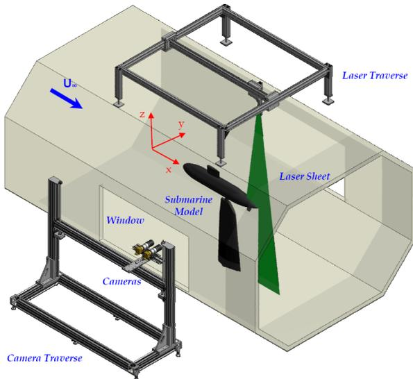
Figure 4. PIV arrangement showing model mounted in LSWT with dual cameras positioned orthogonal to laser sheet
