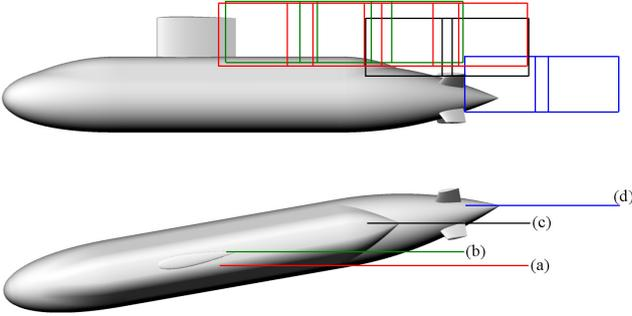
Figure 3. Locations of PIV measurement field-of-view(s) at  $\beta = 10^\circ$  (a) MP1 (b) MP2 (c) MP3 (d) MP4
