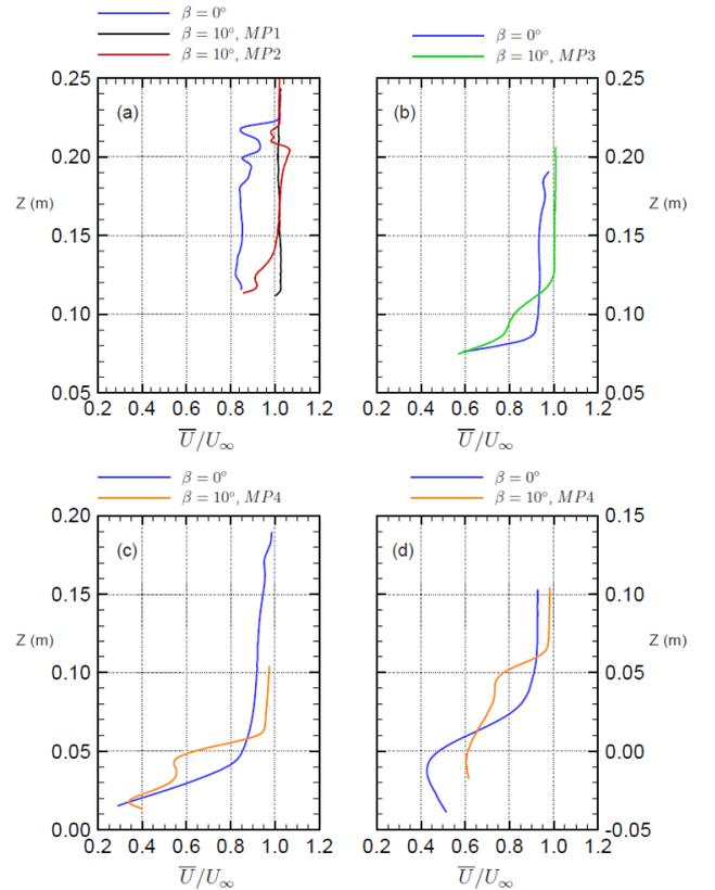
Figure 6. Ensemble-averaged streamwise velocity profiles at (a)  $x/L=0.54$ , (b)  $x/L=0.84$ , (c)  $x/L=0.98$  and (d)  $x/L=1.05$
