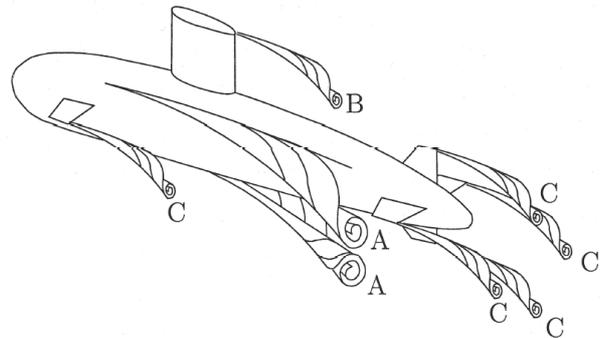
Figure 1. Schematic diagram of systems of vortices generated by a submarine in turn [12]
