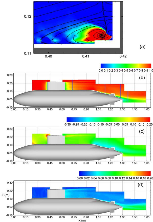
Figure 5. Ensemble-averaged non-dimensional (a) Contours of  $Q$  overlaid with streamlines near the casing-fin junction (b) stream-wise velocity (c) transverse velocity, and (d) RMS turbulence intensity
