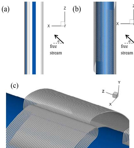
Figure 6. Steady streaming of case of  $KC = 2$ ,  $\beta = 400$  and  $\alpha = 40^\circ$ . (a) eigenvalue  $\lambda_2 = -0.5$ ; (b) streamline; (c) zoom-in view of streamlines.
