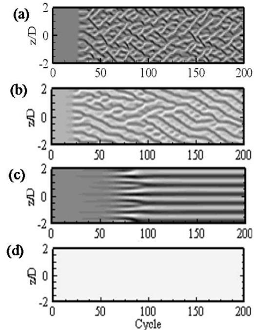
Figure 2. Temporal and special variations of relative axial flow velocity component  $u_z / U_{Mx}$ . Flow development for  $KC = 2, \beta = 400$  at (a)  $\alpha = 0^\circ$ ; (b)  $\alpha = 20^\circ$ ; (c)  $\alpha = 30^\circ$ ; (d)  $\alpha = 40^\circ$ .
