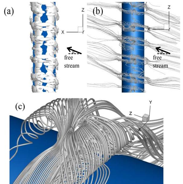
Figure 4. Steady streaming of case of  $KC = 2$ ,  $\beta = 400$  and  $\alpha = 20^\circ$ . (a) eigenvalue  $\lambda_2 = -0.5$ ; (b) streamline; (c) focus of the streamline for one pair of vortical structure.
