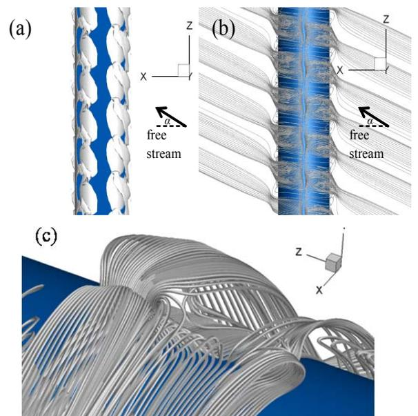
Figure 5. Steady streaming of case of  $KC = 2$ ,  $\beta = 400$  and  $\alpha = 30^\circ$ . (a) eigenvalue  $\lambda_2 = -0.5$ ; (b) streamline; (c) focus of the streamline for one pair of vortical structure.
