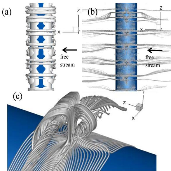
Figure 3. Steady streaming of case of  $KC = 2$ ,  $\beta = 400$  and  $\alpha = 0^\circ$ . (a) eigenvalue  $\lambda_2 = -0.5$ ; (b) streamline; (c) focus of the streamline for one pair of vortical structure.
