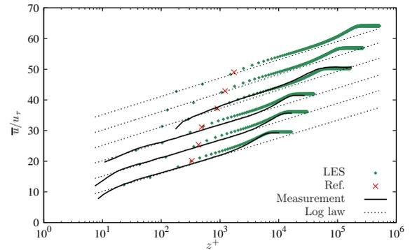
Figure 1: Mean velocity profile for cases 1 – 6 (from bottom to top). The experimental measurements at  $Re_\tau = 7, 300, 13, 600$  and  $19, 000$  are from Mathis *et al.* [9], and that at  $Re_\tau = 62, 000$  is from Winkel *et al.* [16]. Profiles are displaced 5 units of  $\bar{u}/u_\tau$  for clarity. Dashed-lines are log law using dynamically calculated Kármán “constant”.
