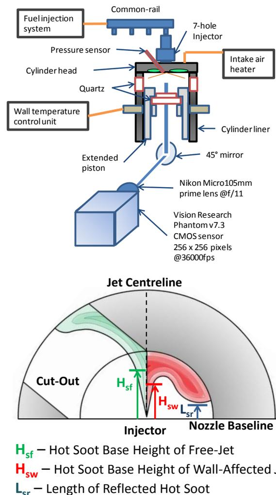
Figure 1. High-speed soot luminosity visualisation setup with a single-cylinder small-bore optical diesel engine (top). A 45° angled mirror located below the chamber provides optical access of the combustion chamber. A sectioned view of the bow-rim cut-out piston shows the separation of jet structures into a free-jet (green, bottom) and wall-affected jet (red, bottom).
