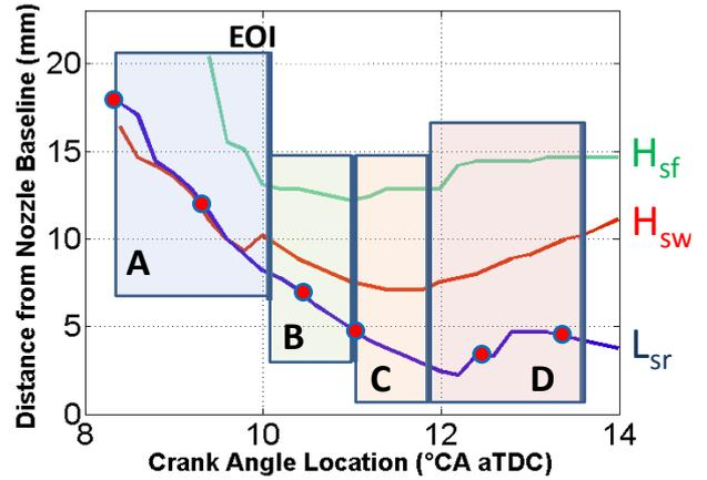
Figure 4. Hot soot base heights for free-jet ( $H_{sf}$ ), wall-affected jet ( $H_{sw}$ ) and length of the reflected hot soot ( $L_{sr}$ ) over various crank angle degrees after the top dead centre (°CA aTDC). Four different events (A~D) are identified from the image analysis of soot luminosity. To illustrate, circle symbols are provided on the  $L_{sr}$  trace for each image time given in figure 3.
