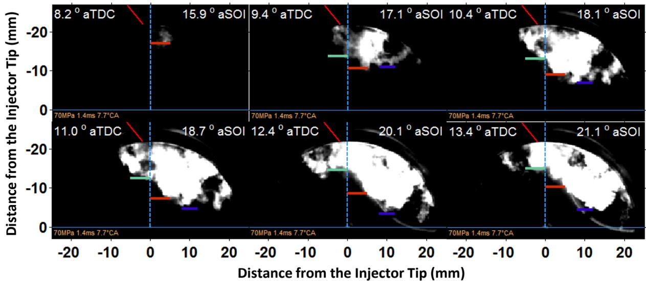
Figure 3. Temporal evolution of soot luminosity from 8.2 ~ 13.4 crank angle degrees after the top dead centre (° aTDC) that corresponds to 15.9~21.1 crank angle degrees after the start of injection (° aSOI). The end of injection occurs at 10° aTDC.
