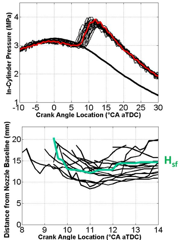
Figure 2. In-cylinder pressure trace of individual cycles (top, black lines) and chosen best representative cycle (top, red line) close to the mean of the variance. Corresponding hot soot base height of the free jet ( $H_{sf}$ ) (bottom, green) is shown amongst the rest of the individual  $H_{sf}$  (bottom, black lines).
