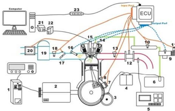
Figure 1- Schematic of the research engine system
