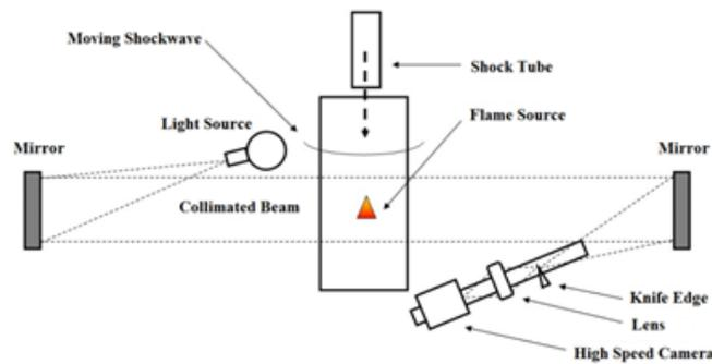
Figure 1. Schematic of the rig and schlieren setup. Not to scale.
