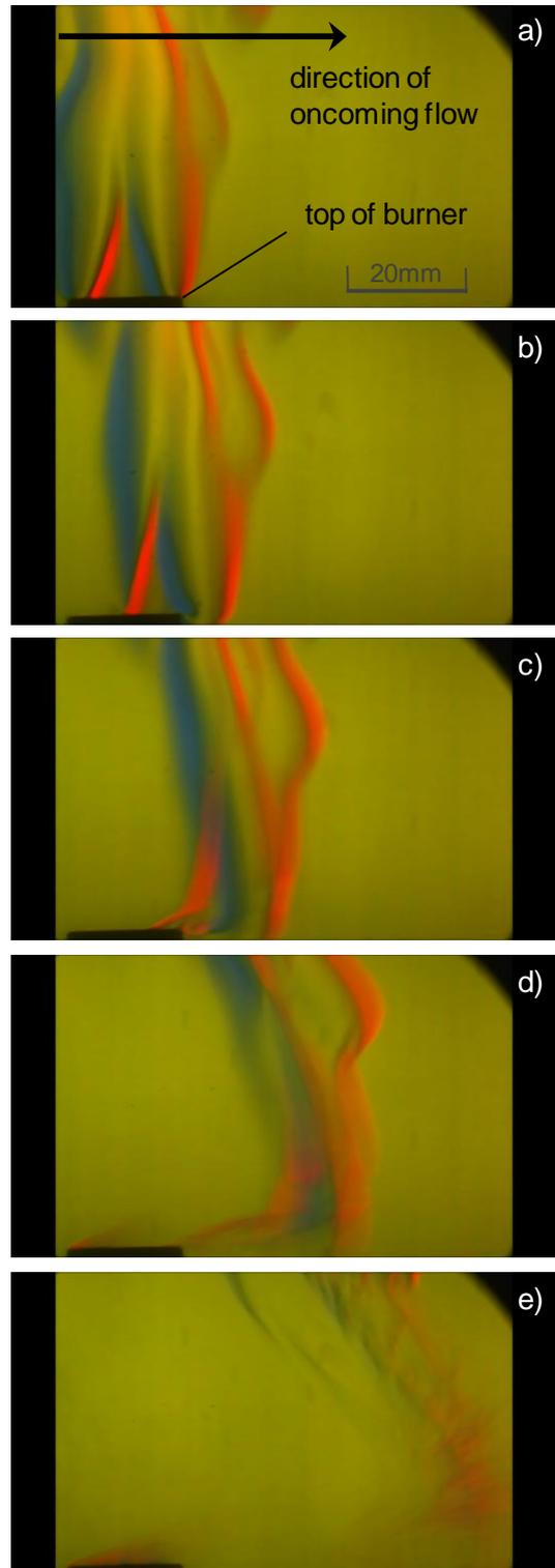
Figure 2. Sequence of frames from high-speed video spanning a period of approx. 0.003s, showing extinguishment of “yellow” Bunsen flame placed 500mm from the shock tube exit.
