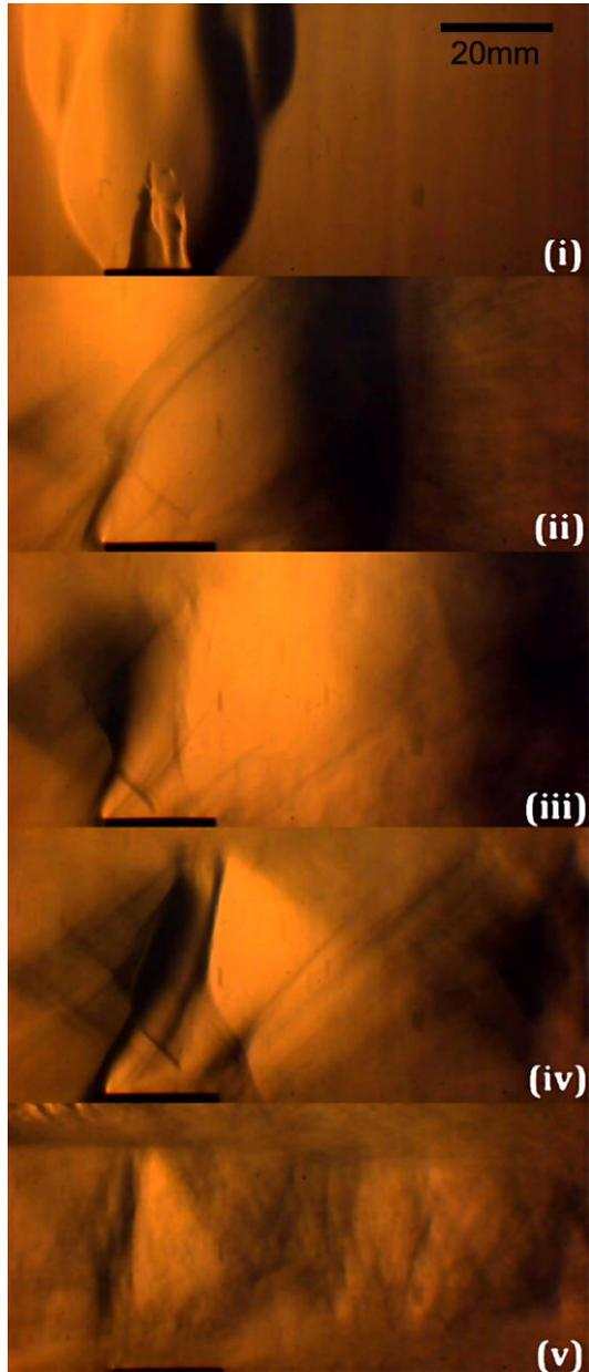
Figure 3. Sequence of frames from high-speed video spanning a period of approx. 0.002s, showing extinguishment of “blue” (hot) Bunsen flame when flame is placed 50mm from shock tube exit.
