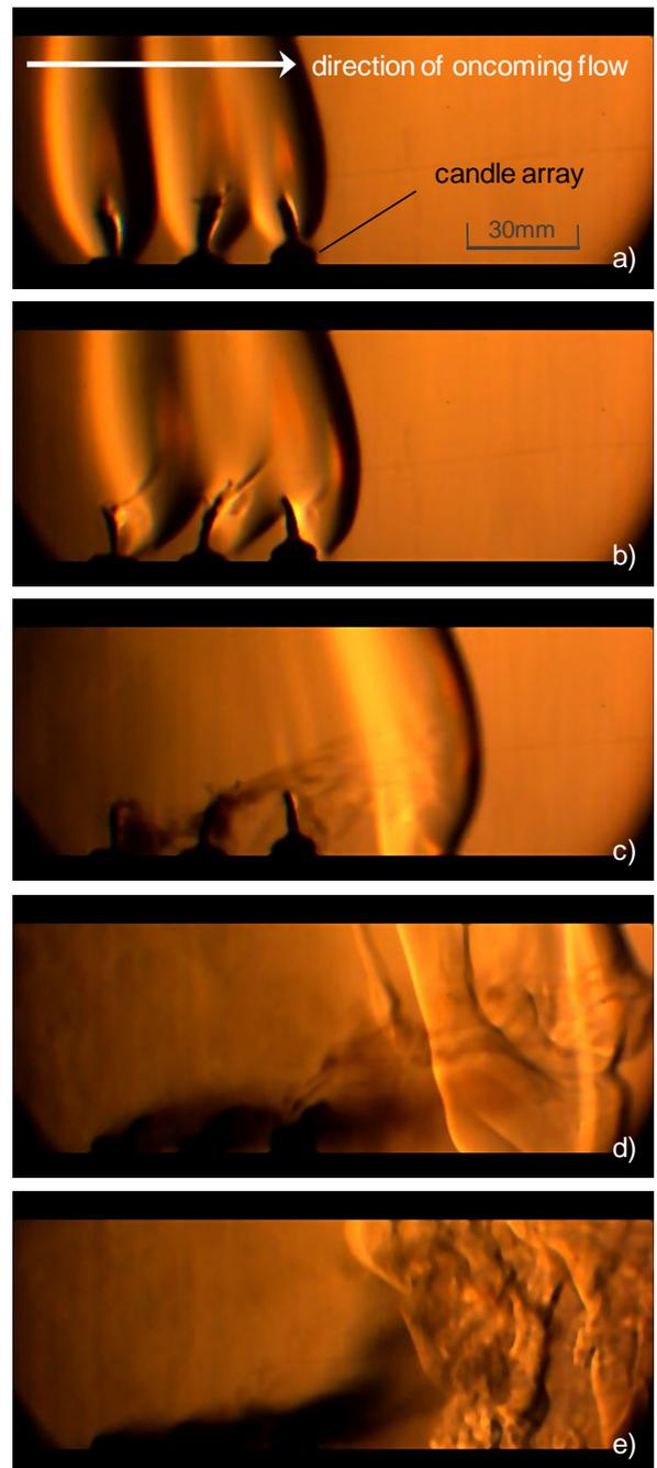
Figure 4. Sequence of frames from high-speed video spanning a period of approx. 0.003s, showing extinguishment of candle array when candles are placed 500mm from shock tube exit.
