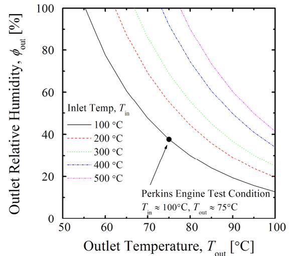
Figure 1. Exit humidity for Diesel exhaust under steady flow condition.
