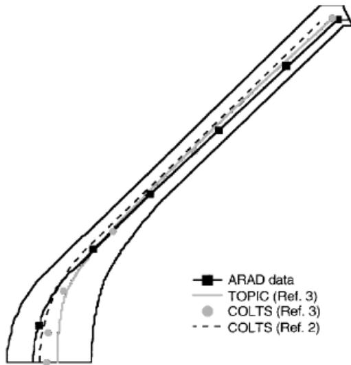
Figure 2: Comparison of the final shape of the Galileo entry probe compared to various theoretical predictions [7]. The solid black line shows the actual surface ablation (with the solid blocks showing where the ablation sensors were located on the heat shield surface), the other 3 lines show results obtained by both NASA and General Electric using two different CFD codes, COLTS and TOPIC.
