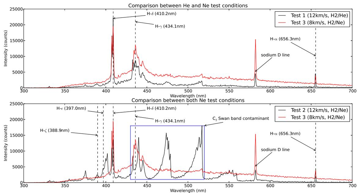
Figure 4: Integrated spectral data from the preliminary test campaign. The top plot shows the comparison between real and substituted gas composition tests, and the bottom plot shows the comparison between low and high speed substituted gas composition tests.
