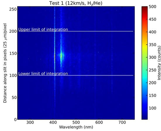
Figure 3: Raw spectrometer data for Test 1. This shows the area integrated over spatially to obtain the data presented in Figure 4.
