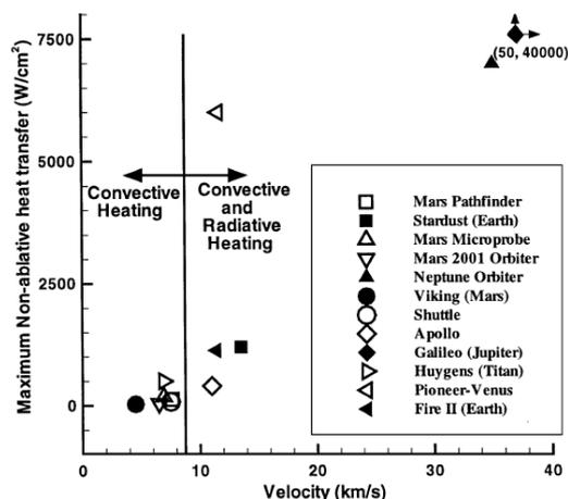
Figure 1: Non-ablative peak heating versus velocity for past and planned planetary entry vehicles [1]. Note the Galileo probe's velocity and maximum heat transfer in the top right hand corner of the plot, and how they're both off the scale.
